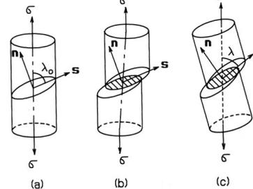
Fig. 10.5 Rotation of crystal lattice in tension
