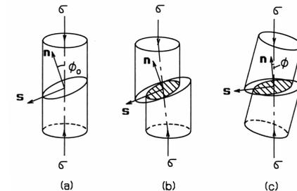
Fig. 10.6 Rotation of crystal lattice in compression
